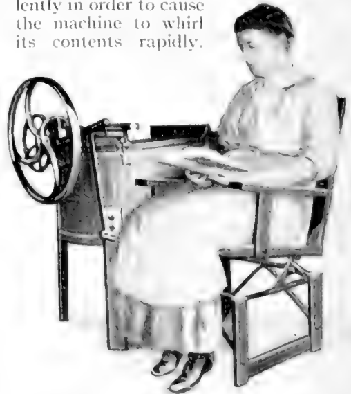
Two springs under the seat of the chair communicate the motion to the washing-machine
